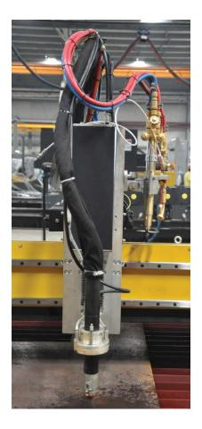
Plasma Torch with Oxy Flame in standby. This is the normal plasma cutting setup illustrating a single torch slide that offers fully cutting width on a high quality linear rail system.
