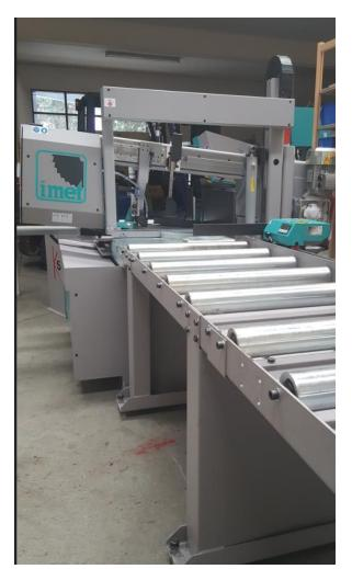
RTL 3KS600- Roller table with 75mm diameter x 600 mm gravity rolls can be used both on loading side and unloading side, with electro welded steel structure, element of 3.0 meters,
